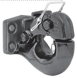
**4.** Push latch closed and insert safety pin, secure pin with spring retainer.
