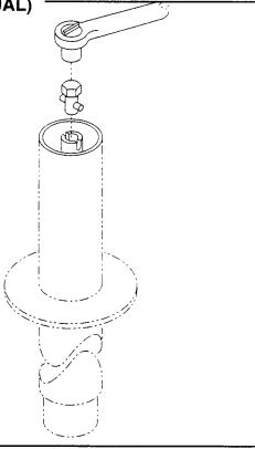
If an electrical failure should ever occur remove the powerhead by loosening the 3 allen set screws holding it to the jackpost. Couple the crank adapter to a 5/8" hex socket, insert into the jackpost and the jack can be raised and lowered.
