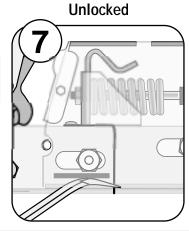
To release the emergency brake bracket, (pictures 6 & 7) insert a brake adjustment tool (looks like a bent screwdriver) into the slot on the release tab (on bottom side of actuator) and pull down until a "click" noise is heard indicating the bracket is released.
