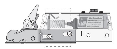
Tie Down's actuators feature a shock dampener that uses brake fluid from the master cylinder. The dampener must be primed before bleeding or using trailer. To prime the dampener, fill the master cylinder with DOT 3 brake Fluid. Push the coupler into the housing and slowly pull out 3 times, then refill master cylinder.
