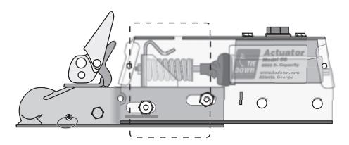
Tie Down's actuators feature a shock dampener that uses brake fluid from the master cylinder. The dampener must be primed before bleeding or using trailer. To prime the dampener, fill the master cylinder with DOT 3 brake Fluid. Push the coupler into the housing and slowly pull out 3 times, then refill master cylinder.
