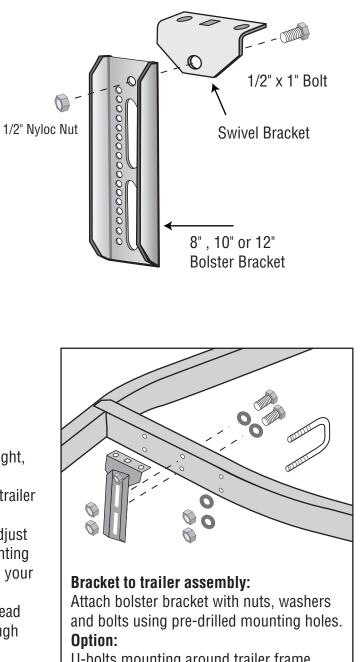
U-bolts mounting around trailer frame. Attach through bolster bracket with washers and nuts.
