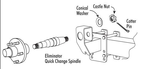
NOTE: Hub & Tire Carrier can be used with any trailer using a 5 lug 1750# UHI Hub, Quick change spindle can only be used with a 3500/3750# Eliminator Torsion Axle.
