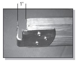
5. Using 3/4" panhead screws, attach corner brackets to the 1x4 stake sides as shown. Center the brackets on the 1x4 extending the bracket out so that there is a 1" gap between the end of the 1x4 and the inside edge of the corner bracket. You will have two long sections (32.5" or 58.5") and two 18.5" sections with corner brackets attached. Diagram below shows proper left and right corner bracket mounting.
