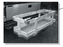
6. Attach the "top layer" 1x4's to the upright 24" posts previously installed. boards should be centered so that there is equal spacing on each end. Boards should be even with top of posts. Use two #8 1-1/4" wood screws at each post. Attach the "long" 1x4's first.
